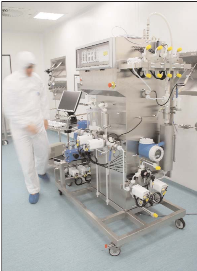
A bioprocess chromatography system in a cGMP suite at Eden Biodesign.
